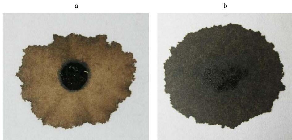
Fig. 4. Photos of the dried drops of the poor quality magnetic fluid and the qualitative one:
