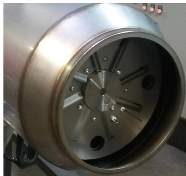
Fig. 4. Flame head of a burner of the 3 rd emission class with a nozzle providing recirculation of flue gases with the formation of the Coandă effect. Gas burner MG3-LN designed by Enertech GmbH Division Giersch (Germany)
