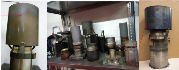
Fig. 3. Various types of caps on the flame tube of the burner to create flue gas recirculation. Photo from the test laboratory of Enertech GmbH Division Giersch (Germany)
