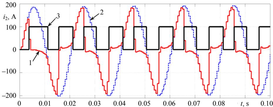
Fig. 6. Saturation detector operation results at  $I_{sc} = 16547$  A,  $\varphi = 90^\circ$ ,  $\tau = 0.065$  s:
