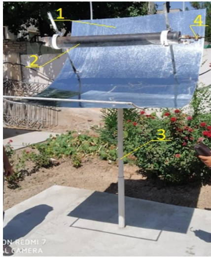
Fig. 3. Heliopyrolysis unit with rotary reactor and solar concentrator:
