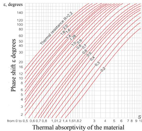
Fig. 4. Dependences of phase shifts on thermal absorptivity of road pavement materials
